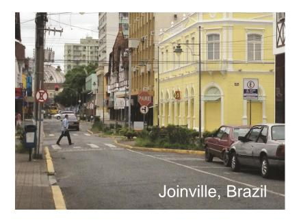
Evidence from Latin American cities shows that the chance of a vehicle collision and pedestrian crash increases by 6 percent for every additional 1 meter of pedestrian crossing distance. Curb extensions are simple ways to reduce crossing distance.
